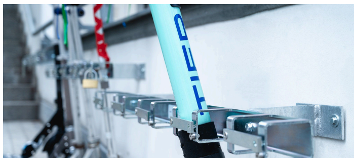
eS Series: Slot 82 x 72 mm, mounting height approx. 60 cm
